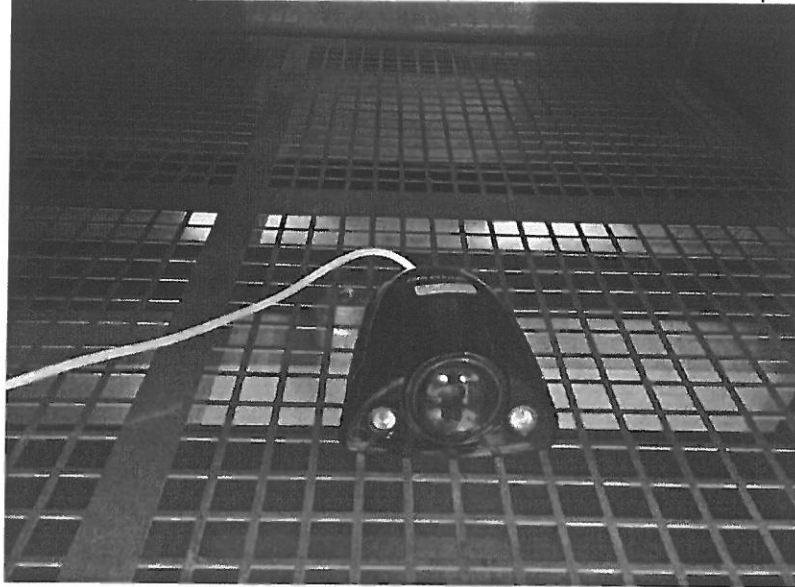
Figure 5: The mounting of the sample in the Environment Test Chamber.
