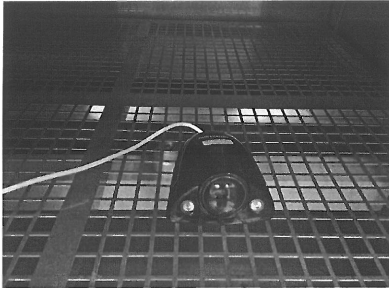
Figure 3: The mounting of the sample in the Environment Test Chamber.
