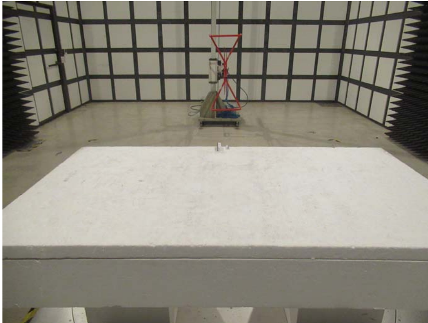
Radiated Emissions- Rear View (Below 1GHz)
