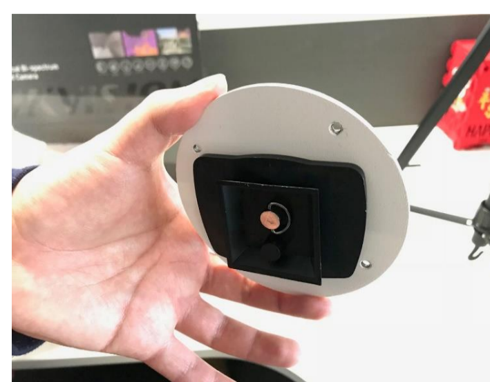
A. Tripod connector fixed on the adapter
