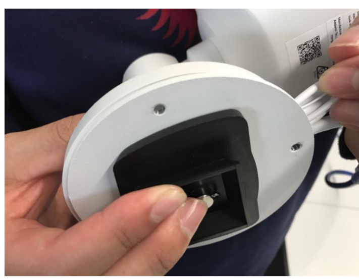
B. Fix the adapter on the camera
