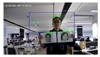
For people coming indoors from cold environment, their skins are with low temperature, which cannot help the device to infer correct temperature. After this low temperature reminder happens, in order to get a valid temperature, measured individuals should stay indoors more than 3 minutes for skin temperature's returning to normal.
