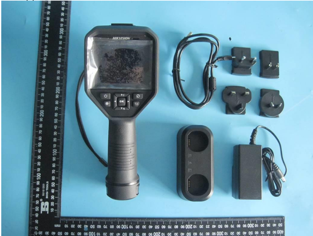
Test item: Handheld thermography camera Tested Model: DS-2TP23-10VM/W
