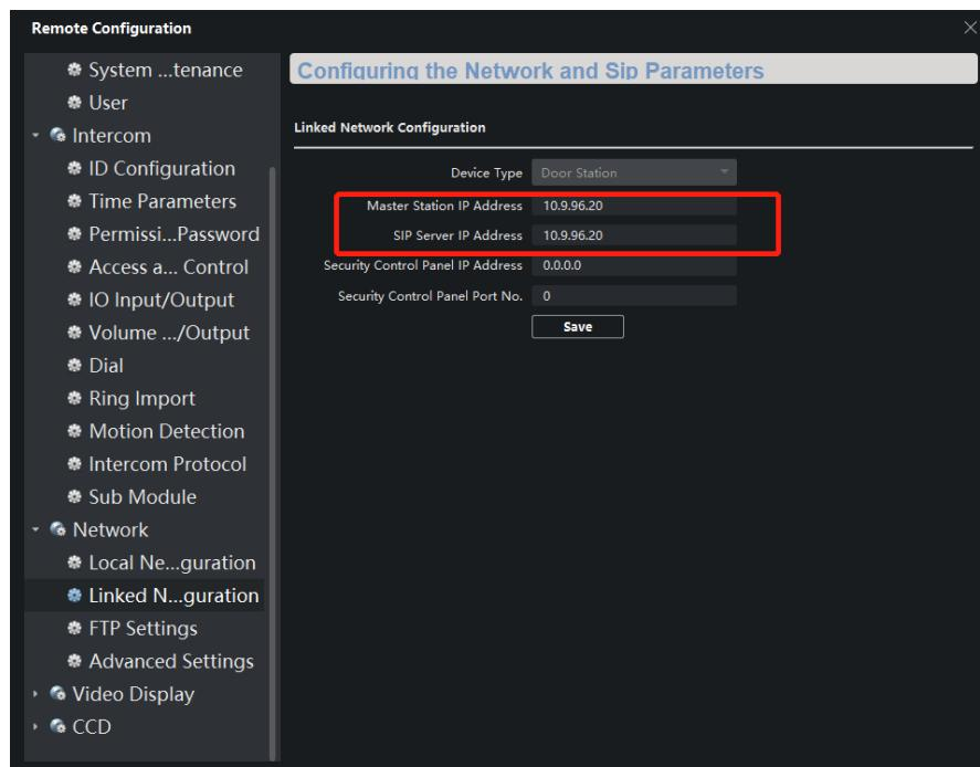
5. On indoor station, input master station IP address to register the indoor station on master station. And input door station IP address to register the indoor station on door station.
