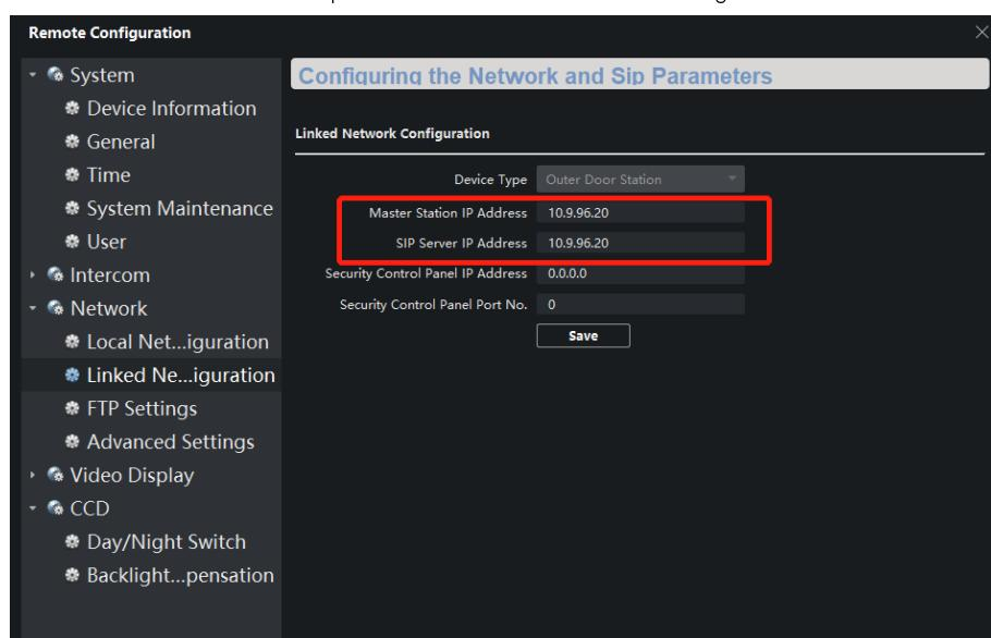
4. On door station, input master station IP address to register the door station on master station.
