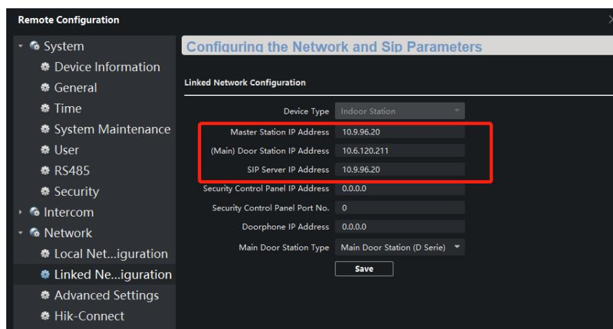
6. On master station, input master station IP address as SIP Server IP Address.
