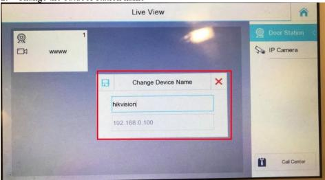
If the indoor station has added the outdoor station, in the live view module, you can see the main outdoor station and sub outdoor station. You can change the outdoor station just press the icon for 2s, then it will pop up a window and you can change the device name.
