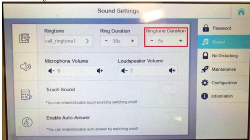
Indoor station can set the Ringtone Duration. By default, the Ringtone Duration time is 5s. It means the ringtone will only last for 5s before it becomes silent. But the call is still on until 30s(Ring Duration) is up.
