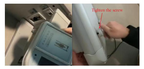
2) After fixing door panel, connect the cable. Right side will be power cable and signal cable, the left side will be signal cable only. Pay attention to the left and right sign and do not make mistake
