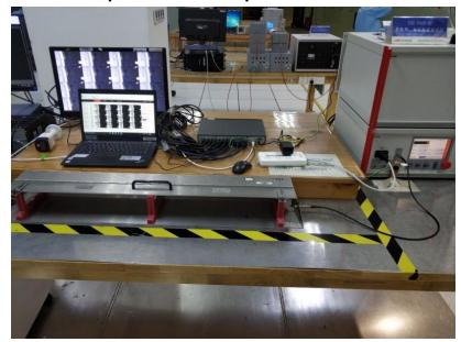
8.15 Mains Supply Voltage Variations-Conditioning Test Setup
