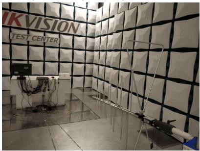
8.4 Radiated Emissions (above 1GHz) Test Setup
