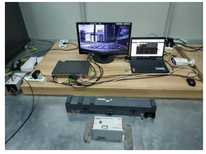
8.13 Conducted Immunity at Signal Port (150kHz-100MHz) Test Setup
