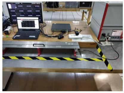
8.9 Electrical Fast Transients/Burst at Signal Port Test Setup
