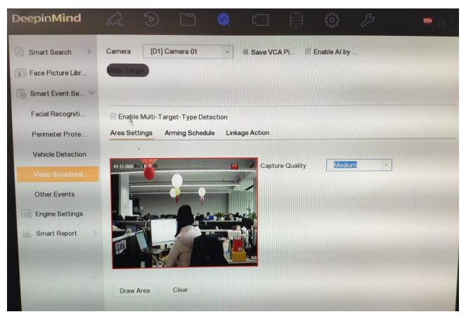
3) Video Structuralization also support the face comparison at the same time. Go to Smart Event Settings > Facial Recognition > Face Picture Comparison and click Enable Face Picture Comparison with the face Librarys needed.(Face capture settings CANNOT be configured in GUI with Video Structuralization engine on)
