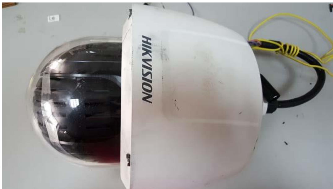
Fig.6 sample1#(after outdoor corrosion test)
