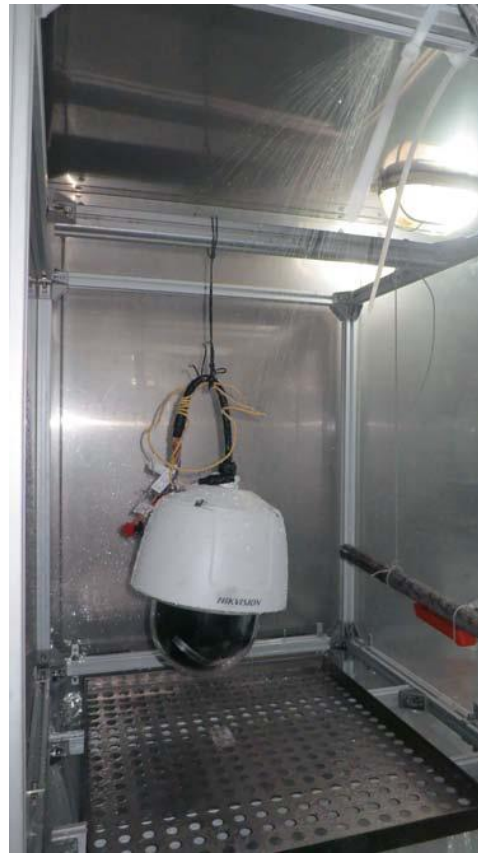
Fig.3 sample1#( during external icing test)
