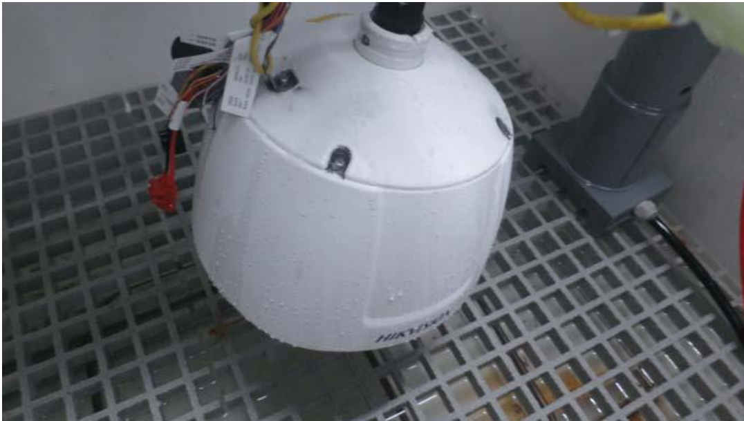
Fig.5 sample1#(during outdoor corrosion test)
