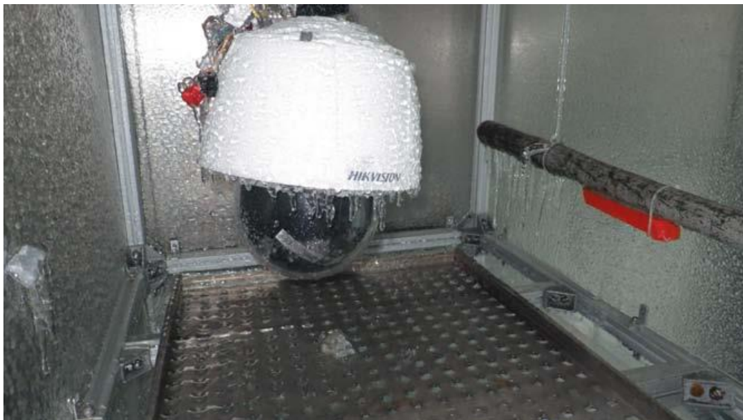
Fig.4 sample1#(after external icing test)
