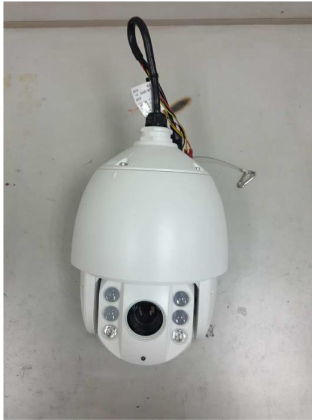
Fig.5 sample1#(After outdoor corrosion test)
