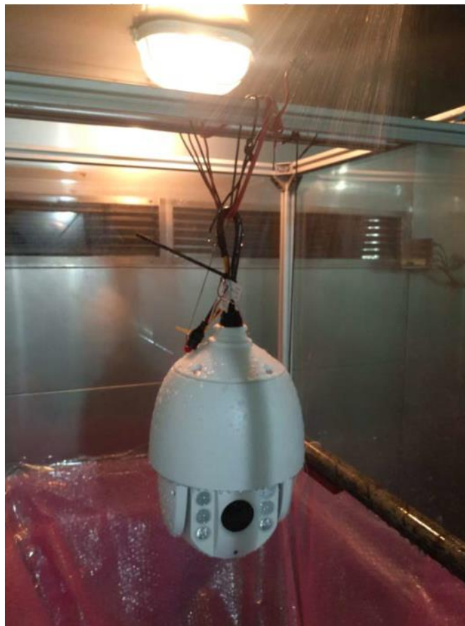
Fig.2 sample1#( during external icing test)
