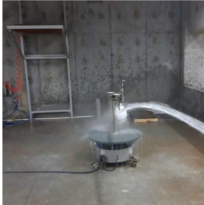
Fig.1 sample1#(during waterproof test)
