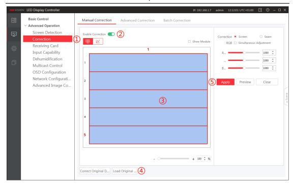
Pls note: every time you change new LED modules, or switch position of the LED modules, calibration will disappear and you will need to operate calibration again
