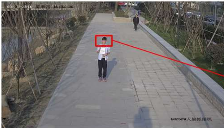
The scenario is too large and the face recognition rate is low
