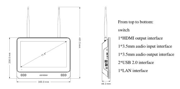
Support a variety of installation methods such as tabletop flat (accessory tabletop bracket) or wall-mounted (accessory includes wall-mounted bracket) to meet the placement requirements of different scenes;
