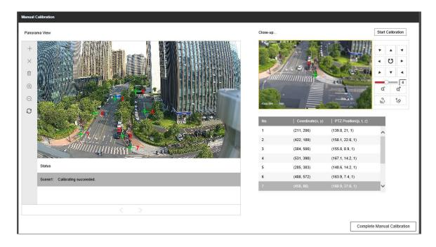
7. After all the coordinates have been calibrated, click Start Calibration on the upper right corner, then click Complete Manual Calibration on the lower right corner. Then this calibration page will exit.
