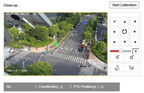
5. After aligning the green cross on both bullet and PTZ channel, click PTZ Position icon to apply the coordination info to the points you just set, then the PTZ Position
