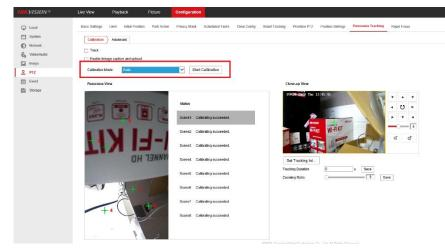
In Calibration Mode, select **Auto**, then click **Start Calibration**. In new window, click **one-touch Calibration**, every scene will do calibration automatically. After all the scenes are calibrating succeeded, click **Auto Calibrating succeeded** to close this window. Also if the picture of scene is old, you can click **regenerate** to capture a new picture for this scene.
