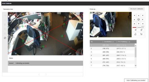
Note: In this application, you can adjust the PTZ camera by pan and tilt button, or you also can use 3D zoom function to set the center of PTZ camera.
