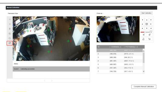
Click Add or Delete icon to add or delete the calibration point, and adjust the position of point by dragging the green cross.
