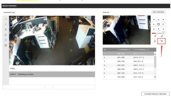
After all of the calibration point adjusted, click the Start Calibration to calibrating, then click the Complete Manual Calibration button to complete the calibration.
