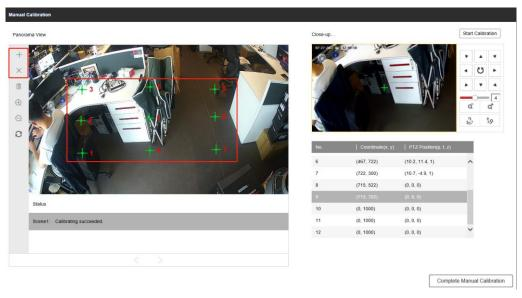
Click the calibration entry in the lower left, and adjust the center of the PTZ camera to coincide with the bullet camera of each calibrate point.
