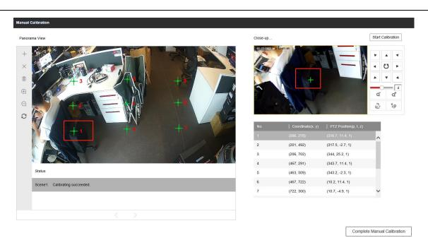
Note: In this application, you can adjust the PTZ camera by pan and tilt button, or you also can use 3D zoom function to set the center of PTZ camera.
