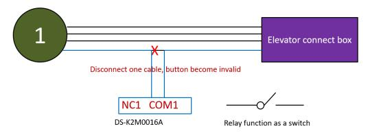
After card/finger/face verified, relay close, floor button recover to default state.
