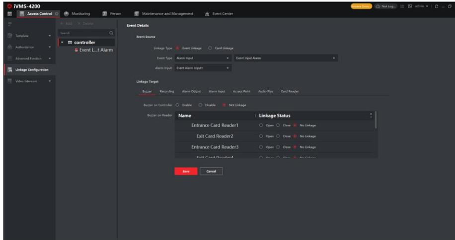
2) You can start configuring the event linkage you need (for example: linkage four doors open) , as shown below.
