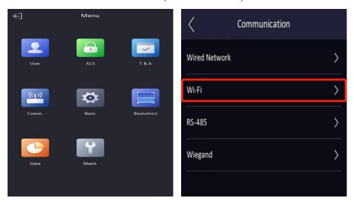
3) Enable the WI-FI and connecting the Wi-Fi.
