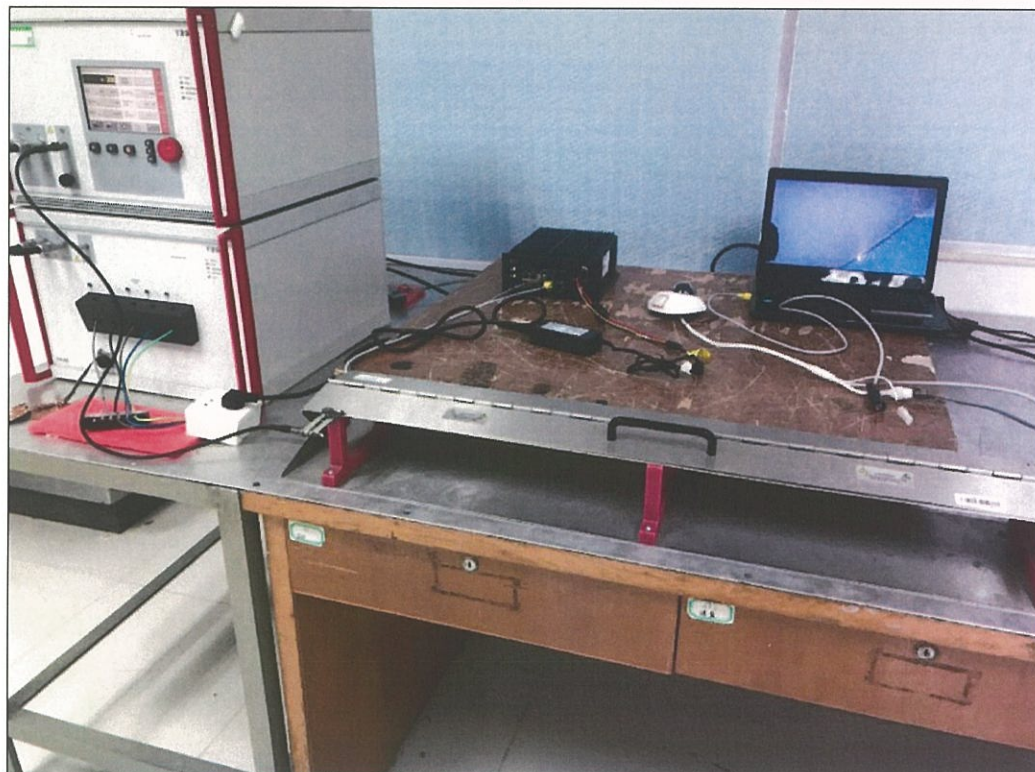
Electrical Fast Transient/Burst Immunity Test Set-Up –Front View(SIGNAL LINE)
