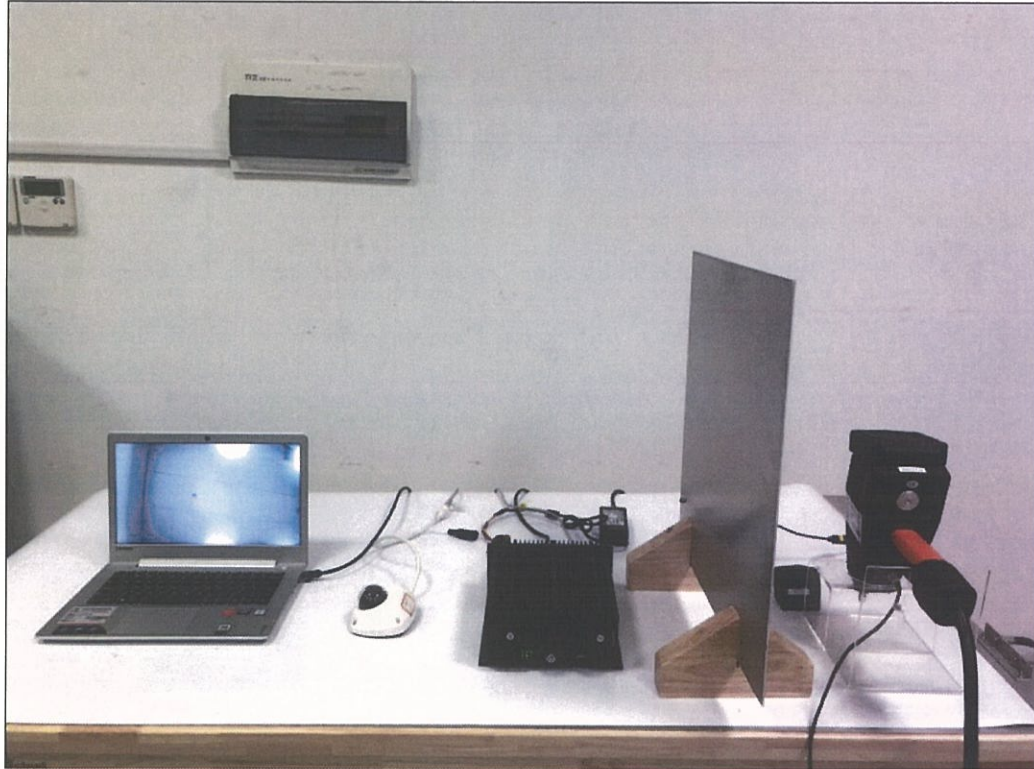
Electromagnetic Immunity Test Set-Up –Front View
