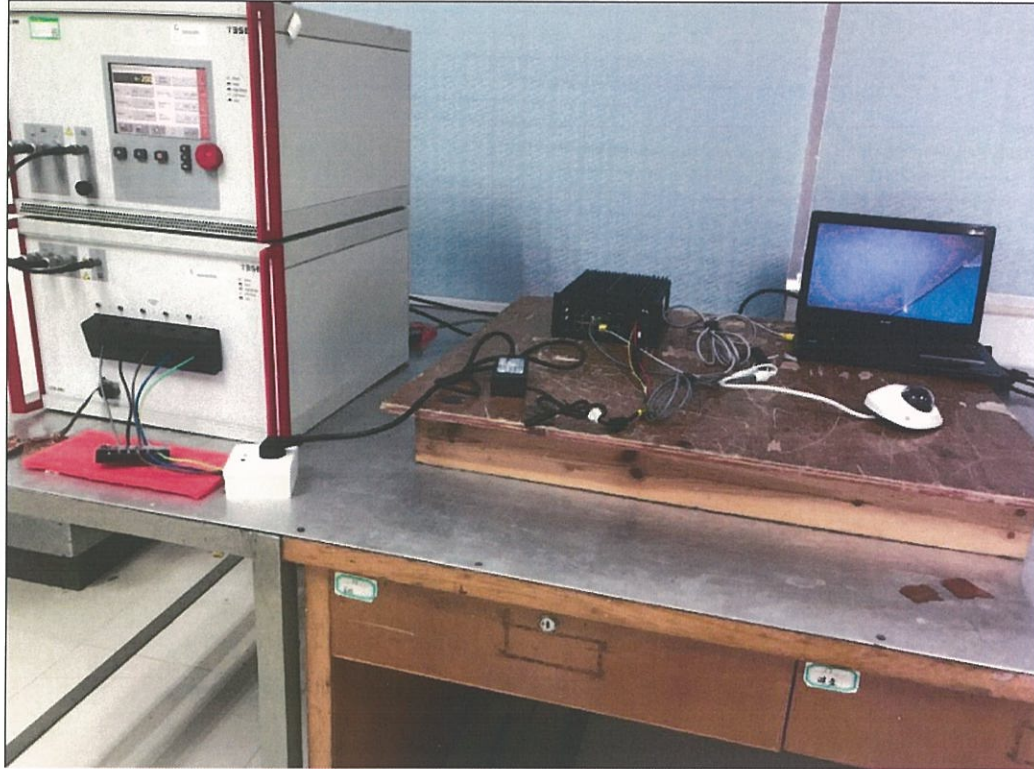
Surge Immunity Test Set-Up –Front View
