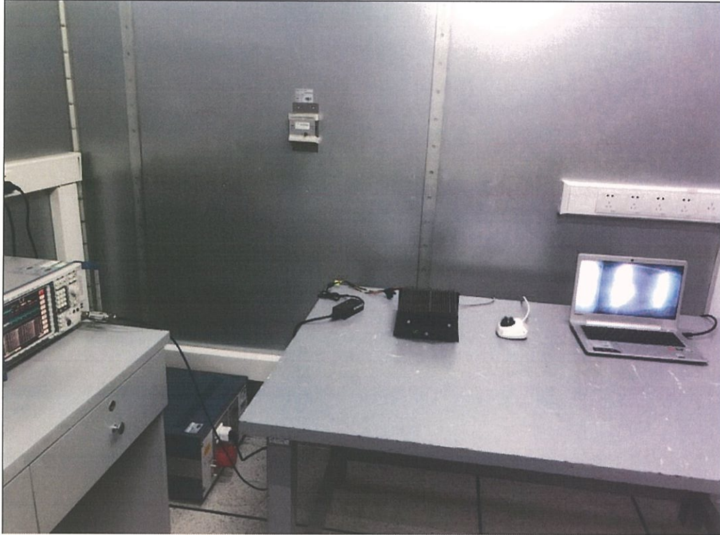
Conducted Emission at mains terminal Test Set-up Front View
