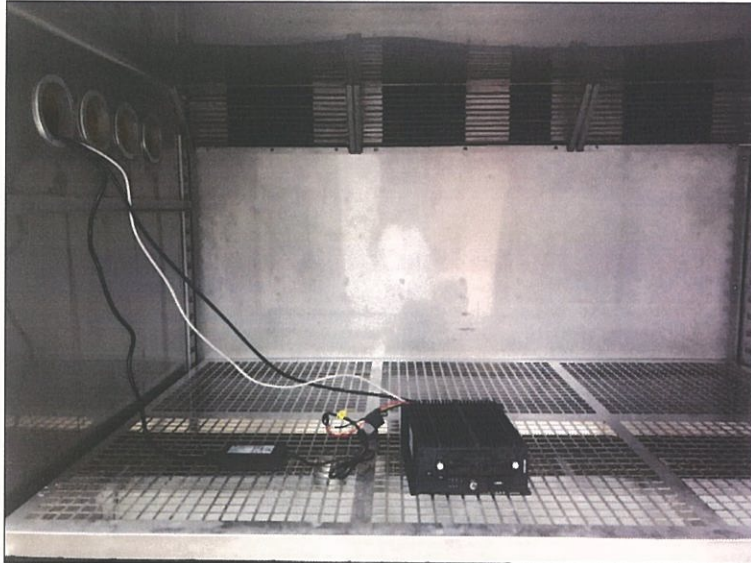
Figure 1: The mounting of the sample in the Environment Test Chamber.
