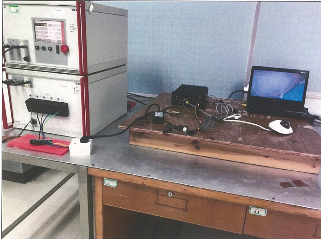
Electrical Fast Transient/Burst Immunity Test Set-Up –Front View(POWER LINE)
