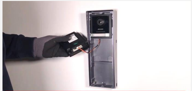
Don't forget to set unique address via the DIP switch of each module
