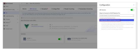
d. Add devices managed on Hik-ProConnect to IP Receiver Pro. In the column of Support Dual-Connection, you will see Yes. This means that you have successfully added a device connected by Dual-Connection.
