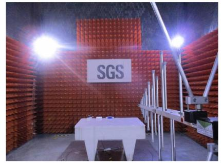
8.2 Radiated Emissions (above 1GHz) Test Setup
