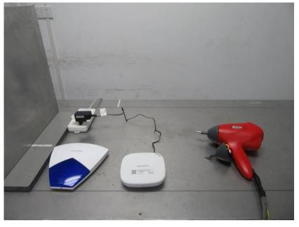
8.4 Radiated Immunity(80MHz-2.7GHz) Test Setup
