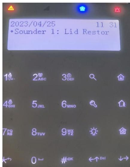
Figure7-4 Area Status enabled and with alarm
