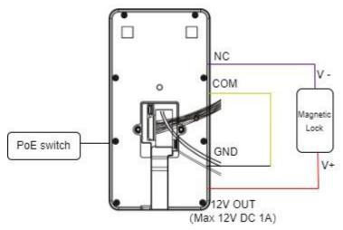
**Note:** Only when device is powered by PoE, it will have power output for the lock, if the device is powered with 12V DC adapter, please power the lock with power adapter.
