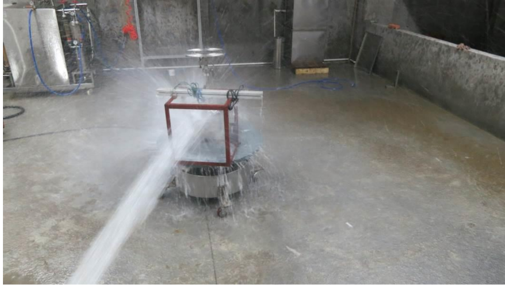
Fig.1 sample1#(during waterproof test)
