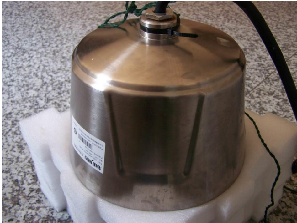
Fig.10 sample1#(after outdoor corrosion test)
