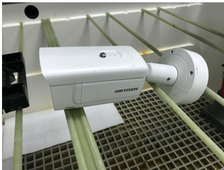
Fig.4 sample1#(during outdoor corrosion test)
