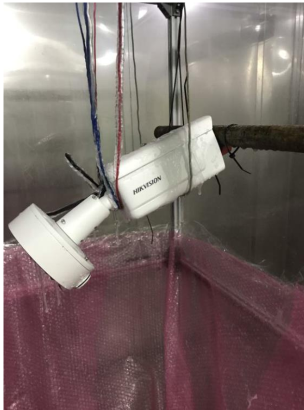
Fig.3 sample1#(after external icing test)
