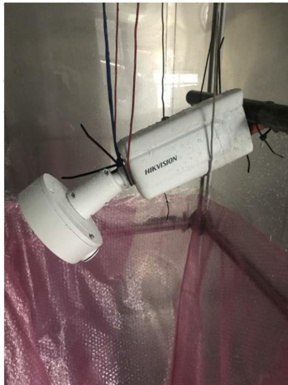
Fig.2 sample1#( during external icing test)
