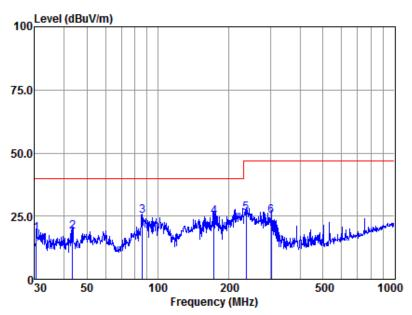
Antenna Polarity :HORIZONTAL EUT/Project :4568IT
