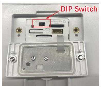
• All the external interfaces of the camera, such as serial port, network cable, SD card, etc., can be used normally after the DIP switch is turned on and the USB power supply is connected.
