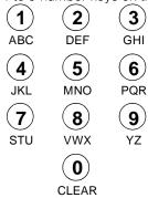
For example, to search for the first zone that begins with the letter "R", press the [6] key three times until the letter "R" is displayed on the keypad between the "< >". Press the [>] key, the first zone that begins with the letter "R" will then be displayed.
