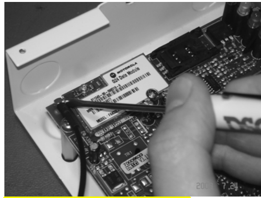
Step 2 - Disconnect existing antenna
