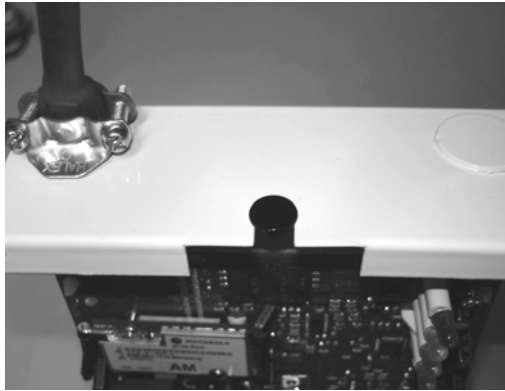
Step 9 - Place plastic hole stud in position
