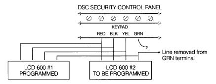
After the LCD's are wired as shown, LCD #2 will have the following message..
