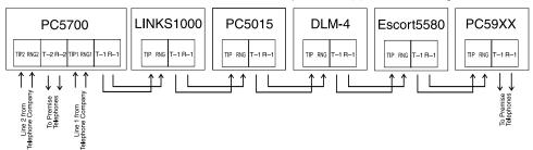
For example, if you are installing a PC5015 with a LINKS1000 and a PC5928 Intercom module, connect the incoming line to the LINKS1000, then from the LINKS1000 to the PC5015, then from the PC5015 to the PC5928 Intercom and then from the PC5928 to the house telephones
