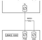
When using the LINKS1000 cellular communicator, any main board zone may be configured for LINKS Supervision. Program this zone as zone type [09], 24 Hour Supervisory in section [001].
