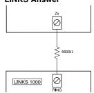
If the LINKS1000 cellular communicator is being used a zone may be configured for LINKS Answer to allow downloading to be performed in the event of phone line failure.
