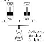
For UL installations, when a bell or siren is used for fire signaling with a pulsed cadence, it must be connected between the AUX+ and BELL- terminals. To maintain bell circuit supervision, do not connect more than one device to the BELL- terminal. A fire bell or siren used for this application must be UL Listed and have a current consumption of 400mA or less (e.g. Wheelock MT-12/24-R).
