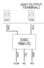
PGM1 can sink up to 50mA of current. Connect the positive side of the LED or buzzer to AUX+, the negative side to PGM1. PGM2 operates similarly to PGM1. If more than 50 mA of current are required, a relay must be used.
