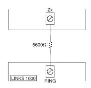
Wire the LINKS Answer zone according to the above diagram. **NOTE:** The LINKS Answer zone is only required for downloading to the panel via the LINKS.
