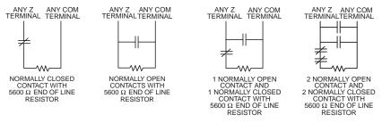
This option can be selected if either Normally Closed (NC) or Normally Open (NO) detection devices or contacts are being used.
