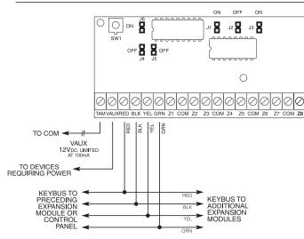
In the above diagram the jumpers settings shown indicate the first group of four zones of the expander will be zones 9 to 12 and the second group of 4 zones will be 13 to 16.
