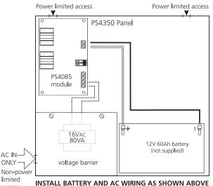
IMPORTANT: A minimum of 1/4" (7mm) separation must be maintained at all points between power limited wiring and all other non-power limited wiring and connections. Wire entry for power limited wiring must be separate from non-power limited wiring.
