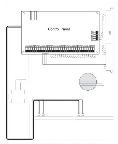
INSTALL BATTERY AND AC WIRING AS SHOWN ABOVE IMPORTANT: A minimum ¼" (7mm) separation must be maintained at all points between battery/primary AC wiring and all other wiring and connections.
