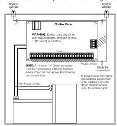
**NOTE:** Wire entry for power limited wiring must be separated by a different entry access from non-power limited wiring.
