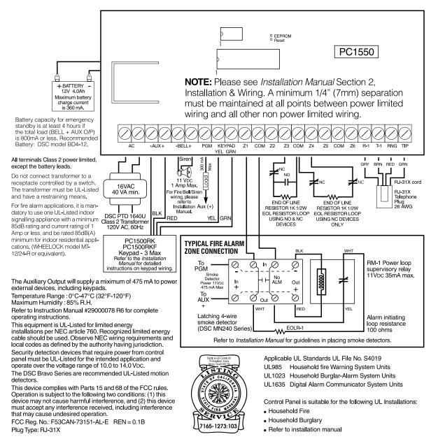
**WARNING:** Not to be removed by anyone except occupant. This equipment should be installed in accordance with the National Fire Code ANSI/NFPA 72 (National Fire Protection Association, Batterymarch Park, Quincy MA, 02269). Printed information describing proper installation, operation, testing, maintenance, evacuation planning, and repair service is to be provided with this equipment.
