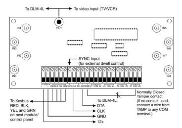
NOTE: If a TV or VCR is used in combination with the DLM-4L, make sure that the jumper J102 on the DLM-4L is removed and the TV/VCR video input is set to 75 ohms.
