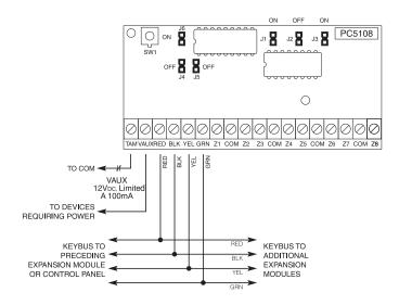
**TAM** - This can be used to tamper the cabinet in which the PC5108 is mounted. Connect a normally closed (NC) switch across TAM and BLK. If the tamper is not being used connect a piece of wire across TAM and BLK to remove the trouble condition.
