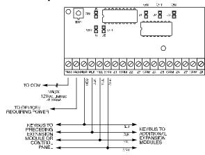
**TAM** - This can be used to tamper the cabinet the PC5108 is mounted in. Connect a normally closed (NC) switch across TAM and BLK. If the tamper is not being used connect a piece of wire across TAM and BLK to remove the trouble condition.
