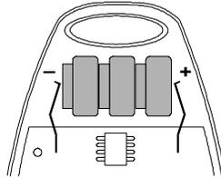
**NOTE: The polarity of the batteries must be observed.**
