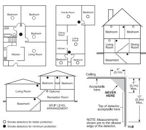
Smoke detectors should always be installed in accordance with NFPA 72, the National Fire Alarm Code and CAN/ULC-S553-02 standard for installation of smoke alarms. Smoke detectors should always be located in accordance with the following:
